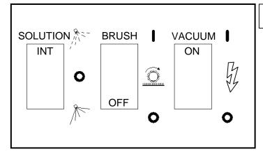
STEP Turn on vacuum motor switch and set solution switch to intermittent position. **Note:** Be sure brush switch is in off position and brush is in storage position.
